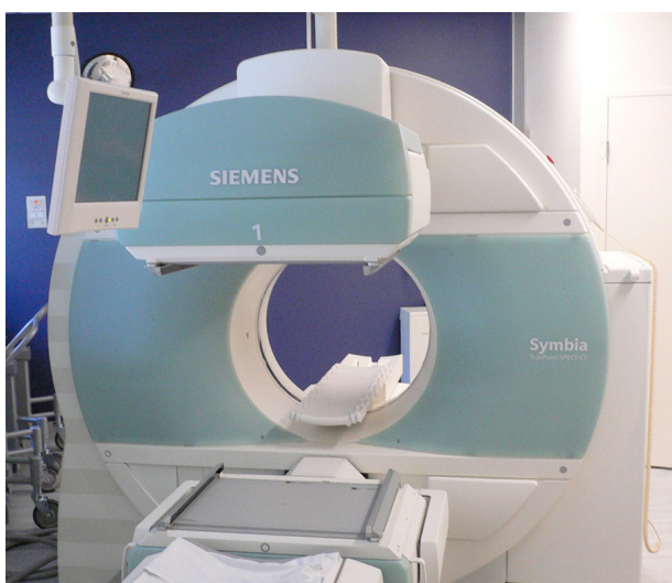
Figure 3 Modern hybrid SPECT-CT scanners incorporate multi-detector CT. This is the Siemens Symbia 6 system installed in these authors' facility.
